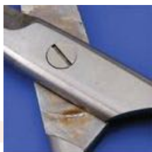
Example of Fretting Corrosion
