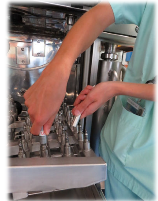
Connexion DHP on LDL rack
