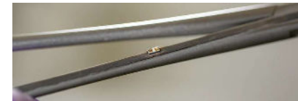
A prototype Smart Tool with an RFID chip and antenna attached to it, allowing for automated surgical tool tracking and counting. Credit: Wyss Institute at Harvard
