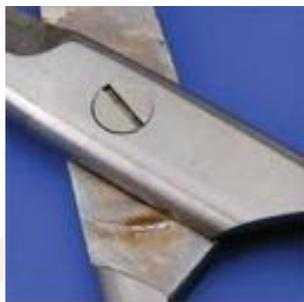
Example of Fretting Corrosion
