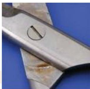
Example of Fretting Corrosion
